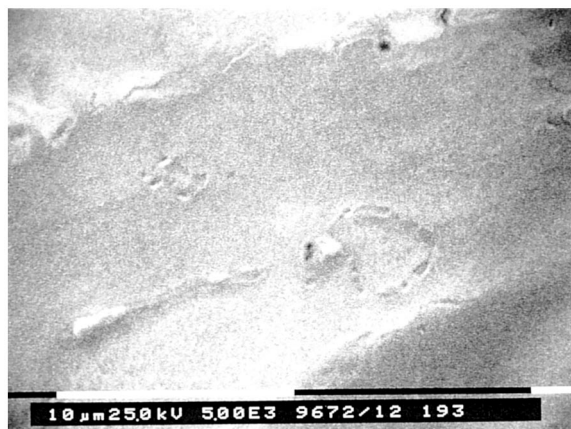
Fig. 6. Homogeneous film of CA pseudolatex observed under SEM.
